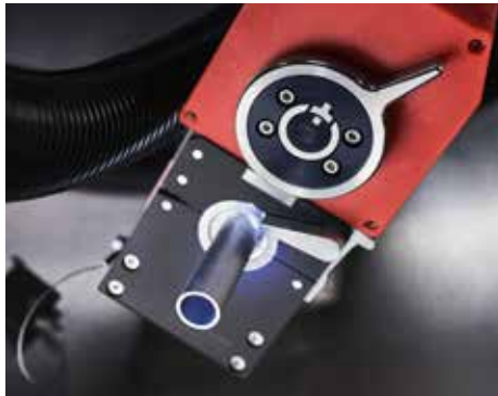
Mico weld head OW 17 GC with clamping cassette
