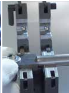
An insertion gage which is permanently attached to the clamping cartridge and thus cannot be lost ensures precise positioning to the tube joint to be welded.
