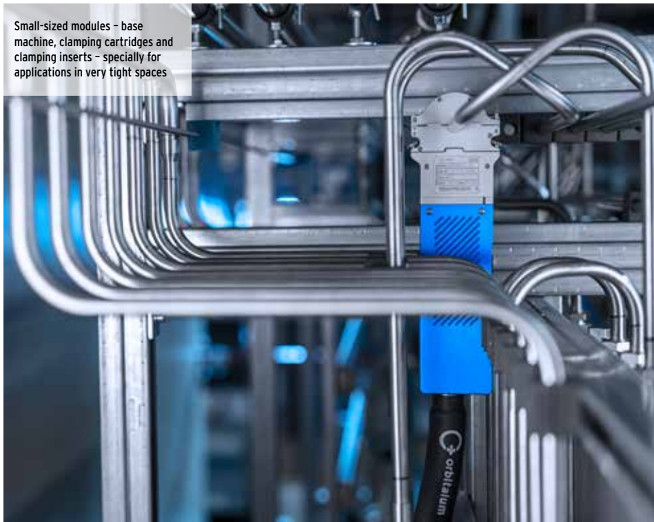
Extremely narrow design and still highly resilient through intensive liquid cooling
