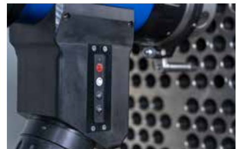
Integrated control panel
