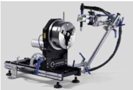
Welding rotary device DVR M
